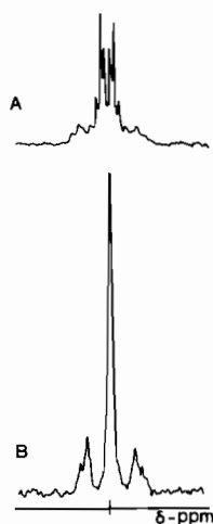
Fig. 2. The imine proton region of the ^1\text{H} NMR (FT, 100 MHz) spectra of [\text{PtCl}_2\text{PBu}_3]_2\text{t-Bu-dim} . a) ^{31}\text{P} and ^{195}\text{Pt} coupled spectrum; b) ^{31}\text{P} decoupled and ^{195}\text{Pt} coupled spectrum.
